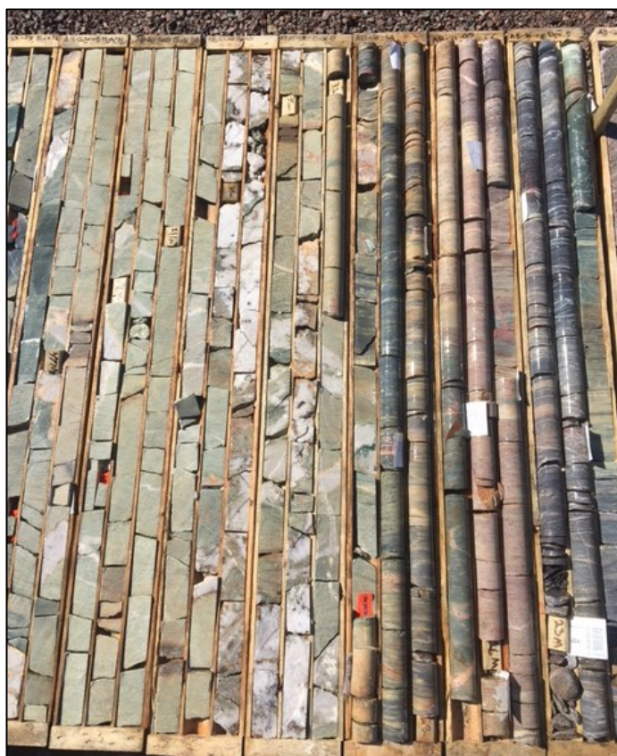
Figure 12.7: Hole AB21-08 - Illite alteration (light green) In Foliated Arkose With White Quartz-Carbonate Veins
