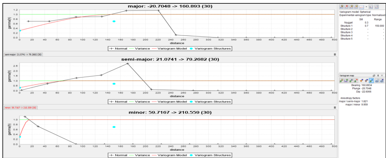
Figure 14.13: Directional Experimental Variogram (Lag 45) of Gold Assay Composites for the Northeast Zone
