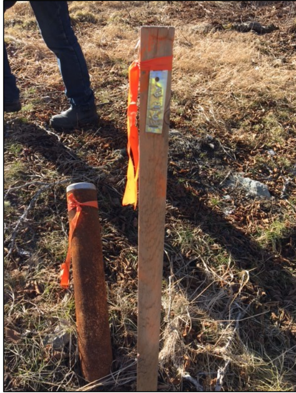
Figure 12.8: Casing and Labelled Picket for Magna Terra Drill Hole AB2021-01
