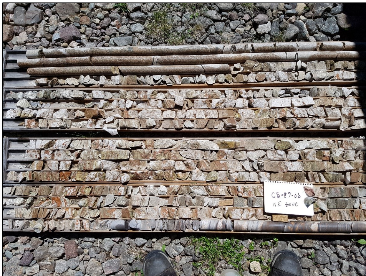
Figure 9.9: Gold Mineralized and Altered Zone in Hole CS-87-06 from the Northeast Zone
