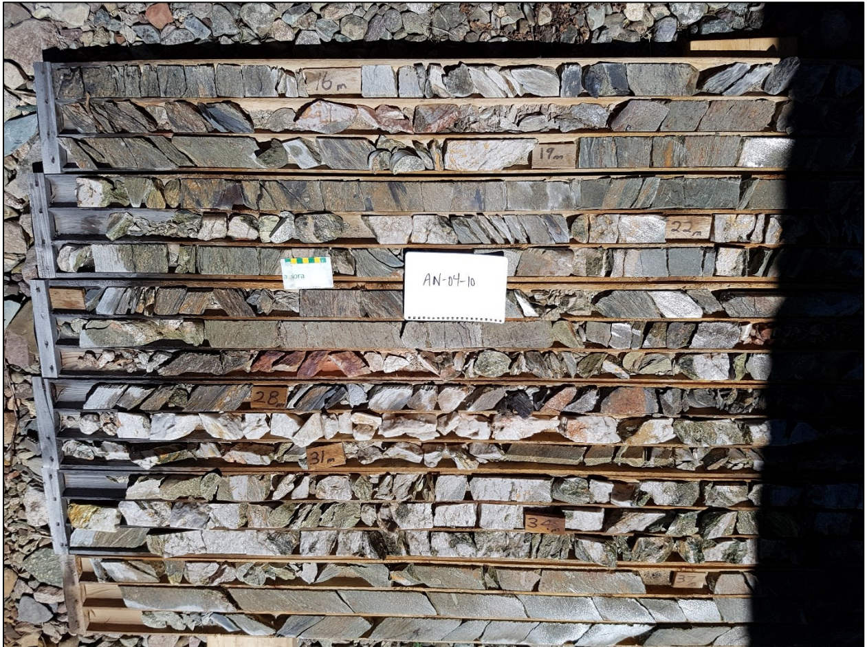
Figure 9.7: Gold Mineralized and Altered Zone in Drill Hole AB-04-10 From Northwest of Pit Zone
